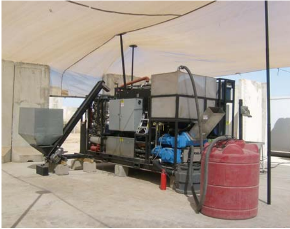
Fig. 6 Material rinsing water routed off the main system through an intermediate sump pump and into a 500 gal tank
