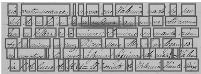
Fig. 9 Word alignment for 6 lines of a particularly noisy part of the corpus. The four last words on the second line as well as the last line illustrate some of over-segmentation and under-segmentation error types.
