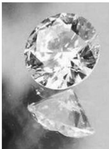
Fig. 9.1 A brilliant cut single-crystal diamond produced from activated low-pressure chemical vapor deposition process [placed on mirror]. Reprinted from S.S. Ho, C.S. Yan, Z. Liu et al. [1] with permission from the Carnegie Institution of Washington
