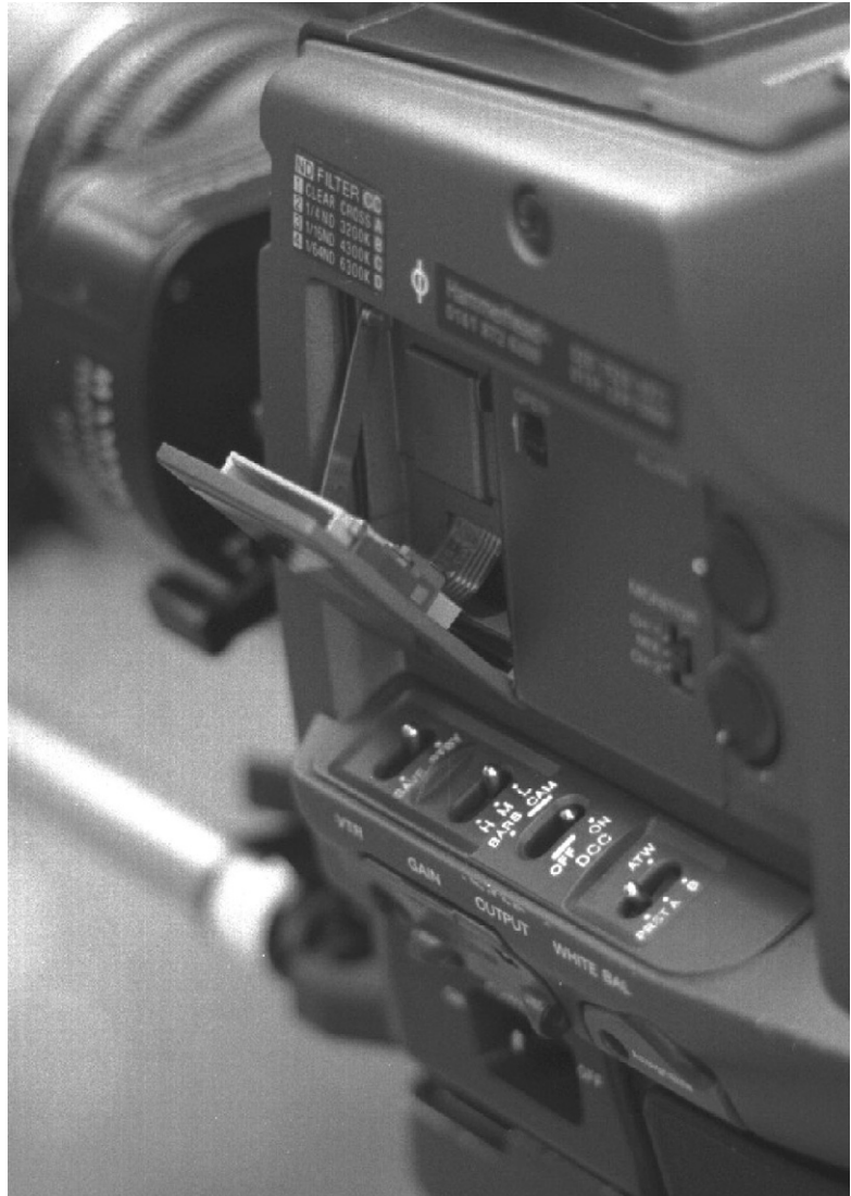
Figure 17.1 Camera control card loading door
