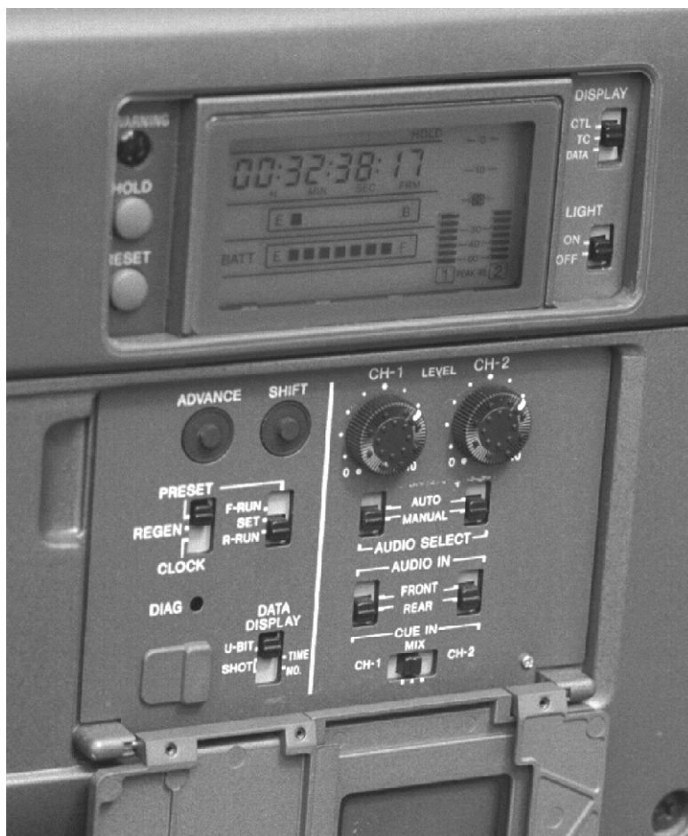
Figure 14.1 Time code and user bits control panel
