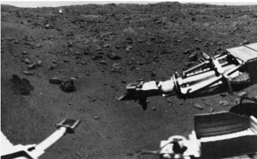
Figure 8.12 Space and planetary teleoperators: (a) the space shuttle arm holding a small satellite; (b) the Viking soil sampling arm on Mars (courtesy of NASA).
