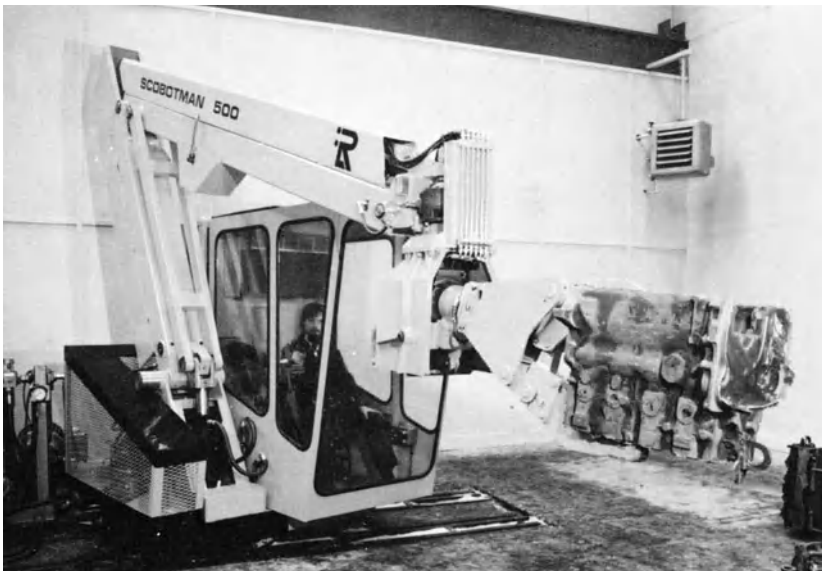
Figure 8.10 Industrial heavy load manipulators: the Lamberton Robotics Scotboman (courtesy of Lamberton Robotics Ltd).
