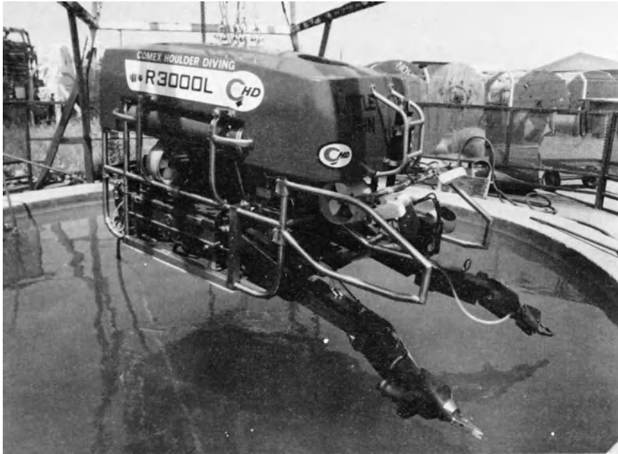
Figure 9.26 An unmanned submersible robot or ROV (courtesy OSEL Offshore Systems Engineering Ltd).
