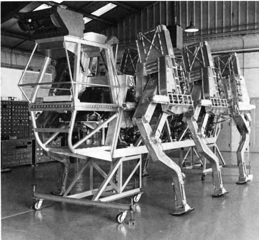
Figure 9.13 The Ohio State University Adaptive Suspension Vehicle (courtesy Ohio State University).
