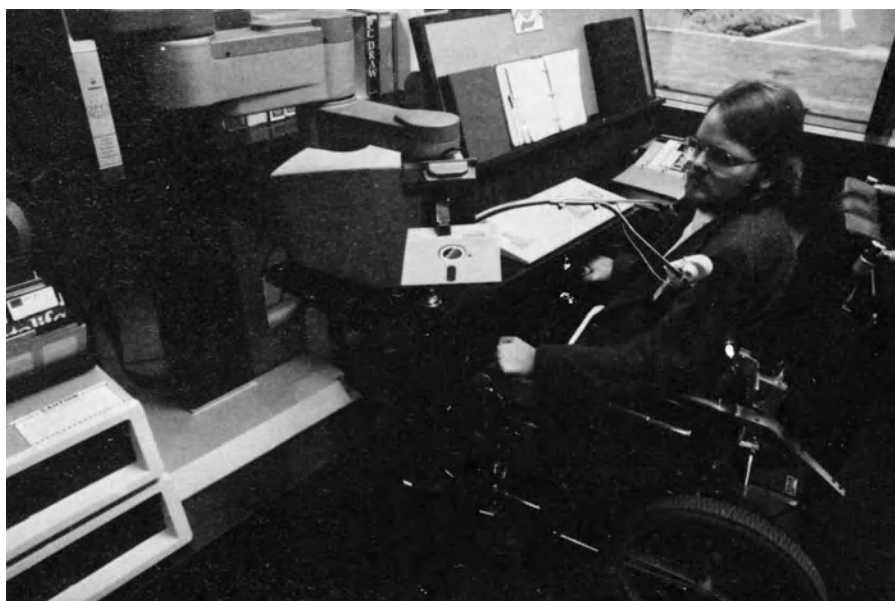
Figure 8.14 An industrial robot controlled as a computer-assisted telemanipulator by a paralyse person (courtesy of Universal Machine Intelligence Ltd).
