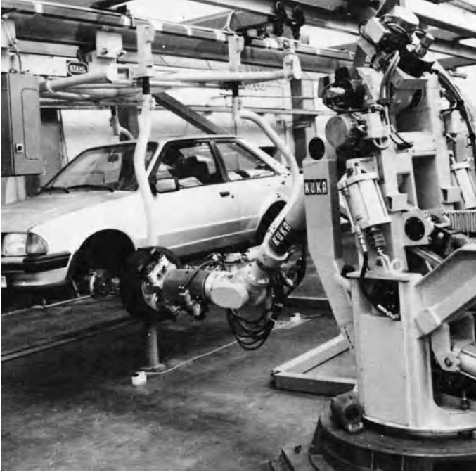
Figure 2.22 A special gripper for holding a car wheel (courtesy of KUKA Welding Systems & Robots Ltd).
