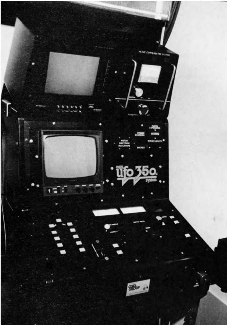
Figure 9.30 The control console for remote operation of the UFO (courtesy of OSEL Offshore Systems Engineering Ltd).
