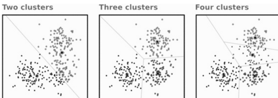
Figure 23.6. Finding the optimum number of clusters for the k -means method. For a given data set, the k -means clustering method can be applied to partition the data into different numbers of clusters. If the number of clusters ( k ) is not known different numbers can be tried so that an optimum can be found. A simple way to evaluate the optimum number of clusters is to measure the relative improvement of the separations of the data points from their nearest cluster centre. Having more clusters will always give smaller separations but there will be the most significant change near the optimum number. For the illustrated example, going from two to three clusters has a bigger jump in minimising separations than going from three to four clusters. Using four clusters only improves separations to the centres mildly.
