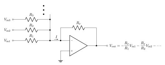
The key to this circuit is that each input voltage and input resistor makes a current; at the big junction, all these currents add and go through the feedback resistor  $R_{\rm F}$ . That is, the total current I is
