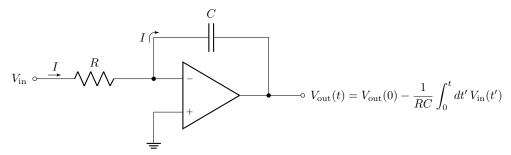
This works more like we said: The input resistor converts the voltage  $V_{\rm in}$  to current I ( $V_{\rm in} = IR$ , with no need for small  $V_{\rm out}$ ), and the capacitor integrates the current to store charge, which produces an output voltage.
