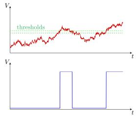
Of course, other nominal trigger levels besides  $0\,\mathrm{V}$  are possible, by replacing the  $1\text{-k}\Omega$  resistor with a voltage divider. The Thévenin resistance of the divider acts in place of the  $1\text{-k}\Omega$  resistor.
