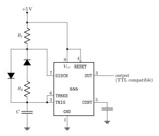
**Solution.** With this arrangement, the capacitor charges through  $R_1$  and the left-hand diode, and discharges through  $R_2$  and the right-hand diode. In either case, we can work out the timing as follows. Suppose the capacitor discharges from voltage (2/3)V towards zero, with time constant RC. We need to solve for the time  $\tau$  when the capacitor voltage is (1/3)V:
