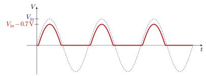
This is not very much like a dc voltage, and not a very good dc power supply. The trick to getting a better dc signal is to add a smoothing capacitor across the load, as in the schematic below.
