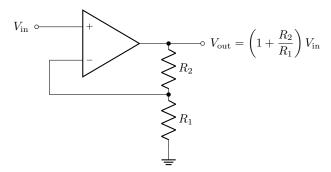
Here, the inverting input sees a source impedance of  $R_1||R_2$ , due to the voltage divider. Thus, it is again a simple matter to insert an equivalent source impedance for the other input.
