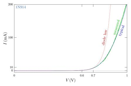
The "diode law" (dashed) curve shows the diode law with  $I_{\rm S}=6.2229\times10^{-9}$  and n=1.9224. The "typical" (solid) curve shows a more complete diode model, which models "high-injection" effects (i.e., the modification of diode behavior due to a high concentration of injected carriers) that become significant on the scale of the "knee current" ( $I_{\rm knee}=43\,{\rm mA}$  here), and a small internal resistance (of about  $0.3\,\Omega$  here).<sup>2</sup> The knee
