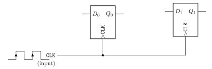
To design the counter, first we will choose the sequence of states that we want. There are no external inputs here, so this is just a simple sequence, with no conditions (which we would represent as extra bits here). The counting sequence is thus as follows:
