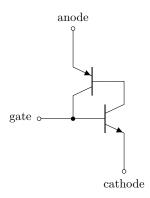
Again, if no current is initially flowing in the circuit, then both transistors are OFF, and no current can flow from anode to cathode, because the current would have to pass via the collector of one or the other transistor.
