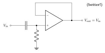
Now, the resistor supplies the path to ground. There is some offset voltage error given by the product of the bias current and the resistance, but this can be made small (in the previous circuit, this error was huge because the impedance to ground was effectively very large).
