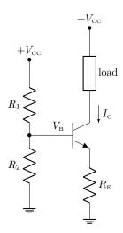
The voltage divider here could even be a potentiometer (variable resistor), so we can fine-tune the regulated current (our treatment is only approximate, for example, because we are using the approximate  $V_{\text{BE}}$  drop of 0.6 V). The voltage divider gives an *unloaded* voltage of
