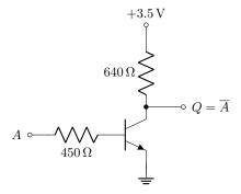
If the input is TRUE, then  $I_{\rm B}>0$ , and the C–E path conducts. This pulls the output down near ground, or FALSE. If the input is FALSE, then  $I_{\rm B}=0$ , and the C–E path is broken. The resistor pulls the output up to the supply voltage, or TRUE.
