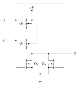
This is a kind of combination of the NMOS and PMOS NOR gates above.  $Q_1$  and  $Q_2$  act as the NMOS NOR gate from above, and actively pull the output LOW if either input is HIGH.  $Q_3$  and  $Q_4$  act as the PMOS NOR gate from above, actively pulling the output HIGH only if both inputs are LOW.
