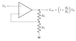
Using that  $R_1$  and  $R_2$  form a voltage divider,
