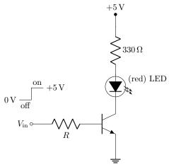
This switch works as advertised (for the stated input voltages) for a resistance R around  $1 \,\mathrm{k}\Omega$ . To learn more about transistor operation, we will consider this resistance and a larger value for the base resistance to see two different regimes of transistor operation. This circuit behaves the same for any of a number of small-signal NPN transistors (2N2222A, 2N3904, 2N4401, etc.).
