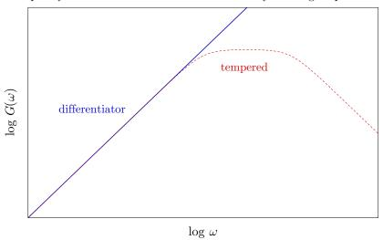
The solid line is the differentiator response, and the dashed line shows the "tempered" differentiator, including the effects of the input resistor (when the gain flattens) and the feedback capacitor (when the gain "rolls off," or decreases).
