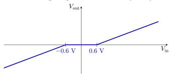
The problem in using this as an amplifier is that it leads to **crossover distortion**, because the base-emitter drop changes as the signal crosses through zero. An example is shown in the graph below of crossover distortion of an input sine wave.
