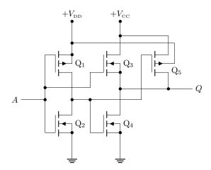
**Solution.** Start with the logic of the first circuit, input A at 0 V.  $Q_1$  and  $Q_2$  form a CMOS inverter, so  $Q_3$  is fed with  $\overline{A}$  ( $Q_3$  0N), and  $Q_4$  is fed with A ( $Q_4$  0FF). This means Q is pulled HIGH, so this is an inverter. Meanwhile  $Q_5$  is fed with A ( $Q_5$  0N). The case with A at  $+V_{DD}$  is similar, but now  $Q_4$  pulls Q LOW, while  $Q_5$  is disconnected.
