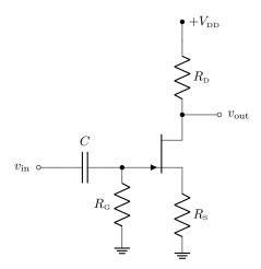
In both cases, the grid/gate is biased at 0 V, and the cathode/source resistor functions to elevate the cathode/source voltage so the grid gate is biased slightly negative with respect to the cathode/source. In the vacuum-tube case, this is called a **cathode-biased** amplifier.
