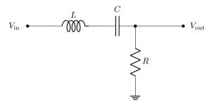
Resonant LC circuits like this are also often called **tank circuits**. To analyze this, let's lump the series inductor and capacitor together into a single element, of impedance
