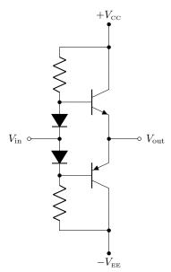
The forward-biased diodes act as part of a stiff voltage divider that set the appropriate bias points; the choice of resistors will affect the impedance seen by the signal source at the input (these could be replaced
