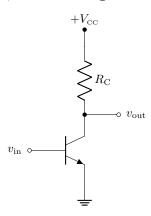
In this case the ac voltage gain is simply the common-emitter gain (4.30) with  $R_{\rm E}$  replaced by  $r_{\rm e}$ ,
