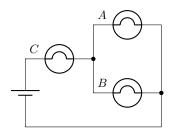
What is the relative brightness of the bulbs? Do bulbs B and C get brighter or dimmer when you remove A?
