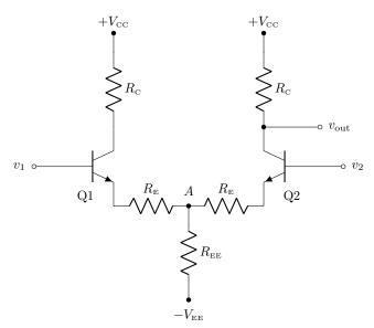
From the layout of the schematic, you can see why this circuit is also called a **long-tailed pair** (the "long" here refers to the magnitude of  $R_{\text{EE}}$ , which as we will see is typically large compared to  $R_{\text{E}}$ ). Note also that the emitter-end of the circuit is powered by a negative supply, so we can have positive or negative outputs.
