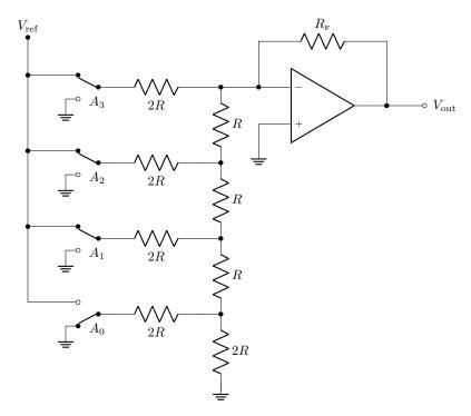
Again, the inputs are  $A_0$ – $A_3$  here, controlling analog/CMOS switches (here SPDT). To see how this works, consider the Thévenin-equivalent circuit for the  $A_0$  input. This is a simple 50% voltage divider, so the equivalent resistance is R, and the voltage is half the input  $A_0V_{\text{ref}}$ . (Note that we consider  $A_0 = 0$  if the switch is down,  $A_0 = 1$  if the switch is up.)
