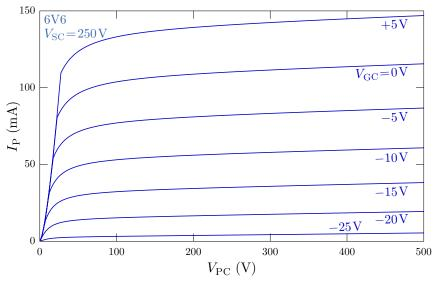
Note that this diagram may be somewhat deceptive, because at small  $V_{PC}$ , the screen voltage is much higher than the plate, and so the screen can attract electrons and develop a substantial current. The figure below superimposes the plate-current curves  $I_{S}$  corresponding to the same gate voltages  $V_{GC}$  (ordered with increasing current in the same way as the plate-current curves).
