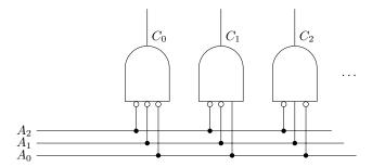
To be more efficient in terms of gates, we would only use one NOT gate for each of  $\overline{A}_0$ ,  $\overline{A}_1$ , and  $\overline{A}_2$ , rather than NOT gates as shown, but the input NOT operations simplify the diagram.
