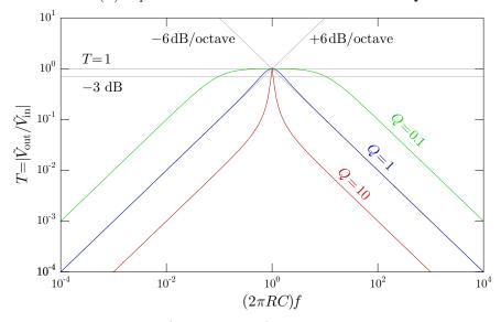
Note that asymptotically, the filter rises/falls at  $\pm 6\,\mathrm{dB/octave}$ , like the low- and high-pass filters.
