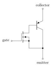
This circuit functions more or less as a BJT, except the C–E conduction is controlled by a voltage  $(V_{\rm GE})$ , rather than a base–emitter current. When  $V_{\rm GE}$  is sufficiently positive, the MOSFET turns 0N, which switches on the PNP transistor and allows current to flow from collector to emitter. Note that in principle this current may flow via either the PNP collector (which is *not* the IGBT collector!) or via the MOSFET drain–source
