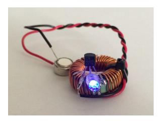
Your exercise here is to trace through the circuit and explain how it works. Just treat the transistor as a switch; no need to do any calculations. Also, as a hint, note that inductors are fairly rare in circuits; usually they show up either as filters (as in the outputs of switching power supplies for computers), or—as is the case here—they are around to give an inductive kick when they are interrupted (like the spark-plug coil in gasoline-powered car engines).
