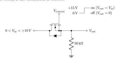
However, for a positive/negative signal, two 2N7000's, back-to-back, are needed for the switch to function properly. Note also that, in the case of the 2N7000, the characteristic curves on p. 145 show that having the ON control signal at least a few V over the maximum possible input voltage is enough to ensure that the MOSFET stays saturated.
