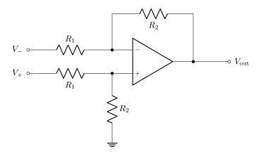
Of course, real resistors aren't perfectly matched. As a model for this, suppose that the feedback resistor has a resistance  $R_2 + \delta R$ , where  $\delta R$  is a small perturbation to this resistance.
