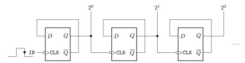
The timing diagram is shown below. Note that we changed the convention for the flip-flops, which now trigger on the *falling* edge of the clock pulse. (Why do we need to trigger on the falling edge? How would you modify the circuit if the flip-flops triggered on a *positive* edge?)
