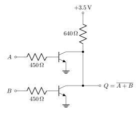
The operation is the same as the NOT gate, but here either input can pull the output to ground; the output is only pulled up HIGH in voltage if both inputs are FALSE or LOW.
