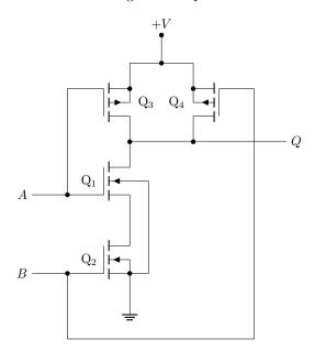
Now  $Q_1$  and  $Q_2$  work together as an NMOS NAND gate, pulling the output LOW only if both inputs are HIGH.  $Q_3$  and  $Q_4$  work together as a PMOS NAND gate, pulling the output HIGH if either input is LOW.
