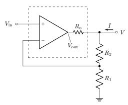
Again, the dashed box represents the "real" amplifier, with an ideal op-amp and the output resistor. We will call the output of the ideal amplifier  $V_{\text{out}}$ , while the "real" output is V. There is also a current I, which we define as flowing *into* the output. Then setting a null input  $V_{\text{in}} = 0$ , we have  $V_{\text{in}+} = 0$ , and now  $V_{\text{in}-} = \eta V$ , so the op-amp rule (7.39) gives
