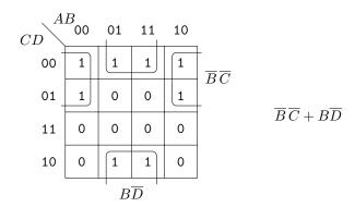
One thing to notice is that we have extended the vertical direction to cover the two variables C and D together, and the other is that we have put in  $4 \times 4$  blocks that "wrap" around from top to bottom or right to left. That is, the Karnaugh map has periodic boundary conditions for the purposes of finding blocks.
