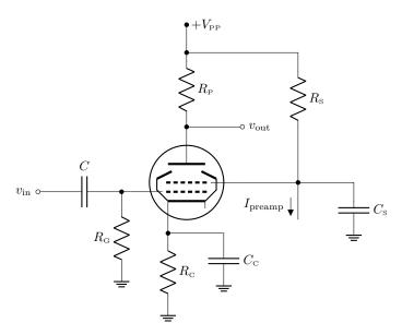
The circuit is similar to the 12AX7 preamplifier before, but now there is a screen resistor  $R_{\rm s}$  that limits the screen current and voltage. A small current  $I_{\rm preamp}$  is also tapped at the screen to power a preamplifier circuit and further drop the screen voltage.
