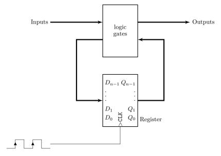
The first main ingredient is a register (Section 13.4.1), which is again an array of D-type flip-flops, with a common clock input. On the rising clock edge, the inputs  $D_j$  are all transferred to the outputs  $Q_j$ , and then held.
