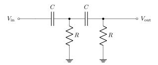
Find the (complex) transfer function  $\tilde{V}_{\rm out}/\tilde{V}_{\rm in}$ , assuming an input frequency of  $\omega$ . How does this scale for large and small frequency? (Also give the scaling at small frequencies in dB/octave.)
