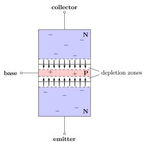
The two depletion zones block any C–E current from flowing (in either direction). Then with voltages set up as  $V_{\rm BE} > 0.6\,\rm V$  and  $V_{\rm CE} > 0$  (actually  $V_{\rm CE}$  needs to be at least roughly 0.2 V), then the B–E depletion zone disappears, and the C–E depletion zone grows a bit.
