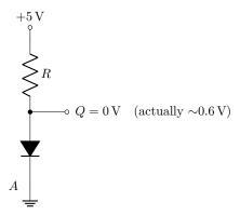
The diode is forward-biased, and thus shorts the output Q to ground. The power-supply voltage  $(+5 \,\mathrm{V})$  is dropped across the resistor because the diode causes sufficient current to flow through the resistor to ground to ensure this. The state of the other input (B) is irrelevant here, because either it "agrees" with A, or if it is HIGH, B's diode is reverse-biased, so it is disconnected from the circuit.
