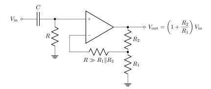
A high-pass filter is used on the input to block the dc component (remember the resistor R is necessary to provide a dc path to ground for the input bias current). We need to balance impedance at dc, so the noninverting input sees a source impedance of R. An easy way to ensure the same impedance for the inverting input is to insert another resistor R in the feedback loop, and simply ensure  $R \gg R_1 || R_2$ , so we don't have to worry about  $R_1$  and  $R_2$  when setting the resistances.
