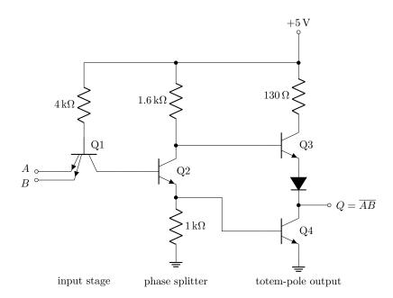
There are three different stages: the input stage (Q1), the phase splitter (Q2), and the totem-pole output (Q3, Q4, and the diode). An unusual feature is the double-emitter input transistor Q1. It works just like a regular transistor, except that a base current to *either* emitter will switch the collector current. Let's trace the voltages through the circuit for two cases.
