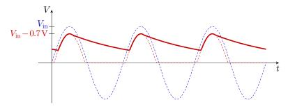
The resulting wave has **ripple**, and choosing the RC time to be as long as possible makes the ripple very small (for good power supplies, the ripple should be of order mV or tens of mV, depending on the current and application). Smaller load resistances (i.e., loads drawing more current) produce more ripple, while larger smoothing capacitors reduce the ripple.
