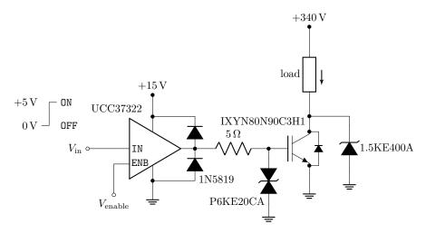
The driver takes a TTL-compatible input (see Section 11.4), but the ON level can also be up to  $+15 \,\mathrm{V}$ . The driver also has an ENABLE input, which forces the output LOW, close to  $0 \,\mathrm{V}$  (this is also true on the inverting UCC37321), independent of the input voltage.
