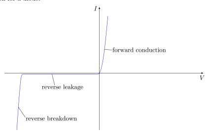
This is the forward current I plotted against the forward voltage V; negative values of course indicate that the voltage/current are going in the reverse-biased direction. There are a few features to notice here.
