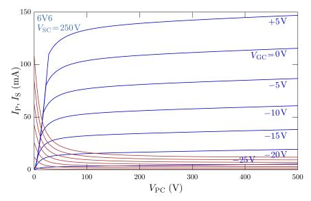
The screen current can be substantial in such a tube, but the screen is a relatively delicate device compared to the plate. For this reason, these tube circuits often employ a resistor to limit the screen current to protect and prolong the life of the screen.
