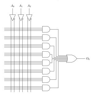
The main grid of lines is intended as a configurable grid, where we can make whatever connections we like. Then there are two ways to think of this. First, because the inputs go first into AND gates and then into an OR gate, we can realize Boolean-logic expressions if they are **sum-of-product** expressions. For example, we can realize
