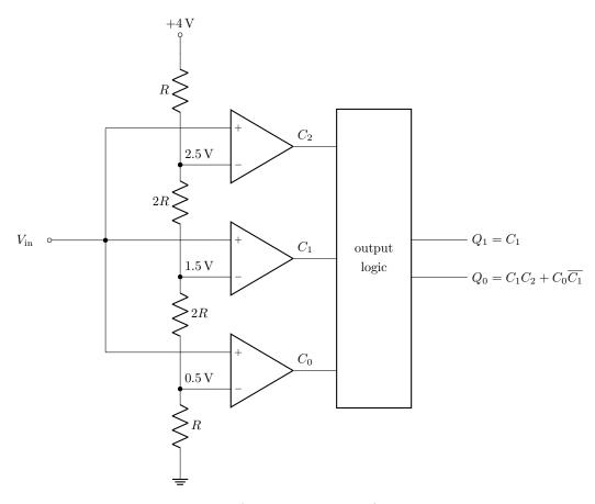
The idea is to choose digital voltage levels ("quantization level") of 0, 1, 2, and 3 V. Then the maximum input range is -0.5–3.5 V with a maximum error of 0.5 V. Then the conversion ranges with comparator outputs are enumerated below.
