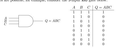
The idea is a reasonable obvious generalization of the 2-input AND: the output is TRUE only when all inputs are TRUE.
