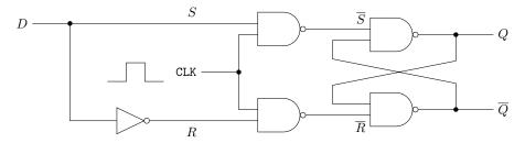
An RS flip-flop (with momentary-low inputs) has two extra gates on the inputs and a clock signal, so that the flip-flop only accepts input from the data line D when  $\mathtt{CLK} = \mathtt{HIGH}$ . The clocked version of the flip-flop is essential in scalable memories. We will actually refer to a modified version of this circuit, shown below.
