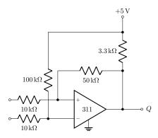
(b) Show how to add another (311) comparator to also produce the  $\overline{Q}$  output. (Use whatever resistors you like.)
