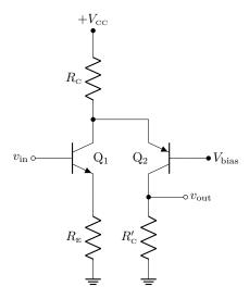
That is, this circuit behaves fairly similarly to the common-emitter amplifier, but with two transistors instead of one (functioning something like a common-emitter amp cascaded with a common-base amp). The main advantages of this circuit are that it suppresses the Miller and Early effects.
