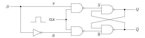
The idea is that there is now only one input, and the flip-flop latches the value of the data while CLK is HIGH. This flip-flop is often called a **data latch**.
