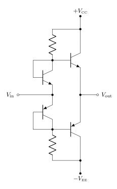
This better matches the bias voltages to the base–emitter drops, but is probably only practical for signal-level circuits (this is a common trick in the internals of an op-amp, for example).
