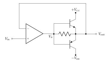
This circuit acts as a unity-gain buffer with high current-driving capacity, because the op-amp does whatever it needs to do to ensure that  $V_{\text{out}}$  is the same as  $V_{\text{in}}$ . And to do this, it must "undo" the crossover distortion, so the base voltage  $V_{\text{B}}$  in this circuit must respond to the input as in the graph below.
