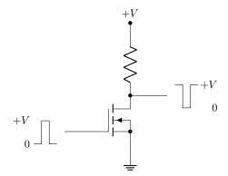
This behaves in much the same way as the RTL NOT gate of Section 11.3.2. With zero input voltage ( $V_{GS} = 0$ ), the MOSFET behaves as an open switch, so the output gets pulled up via the resistor to +V. With a positive input voltage, the MOSFET acts as a closed switch, so the output is actively pulled close to ground.
