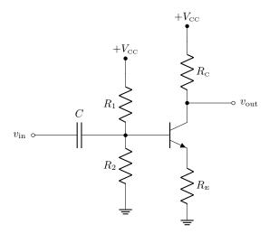
Here, the voltage divider sets the bias voltage, and the input capacitor only passes the ac part of the input signal.
