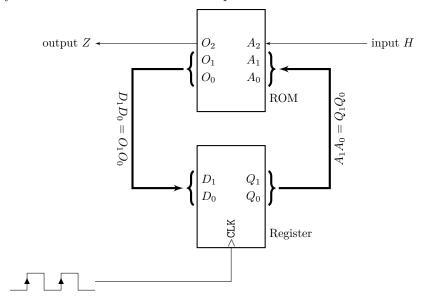
All the logic in the truth table, of course, must be programmed into the ROM. Thus, for example, in address  $A_2A_1A_0 = 000$ , corresponding to  $HQ_1Q_0 = 000$  in the truth table, we simply program in the value  $D_1D_0Z = 011$ , and so on for the rest of the 8 total memory locations.
