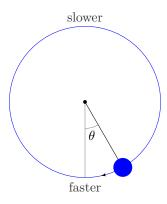
Because the kinetic energy is lower when the pendulum is going "over the top," the angular velocity is lower at the top than at the bottom. In the phase-locked loop, this means  $|\Delta\dot{\phi}|$  is larger when  $\Delta\phi$  is near  $0, \pm 2\pi, \pm 4\pi, \ldots$ , while it is smaller when  $\Delta\phi$  is near  $\pm \pi, \pm 3\pi, \ldots$  We can model this by writing (assuming  $\Delta\dot{\phi} > 0$ )
