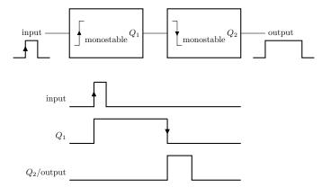
Note the different edge triggers of the two monostables.
