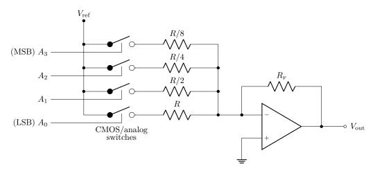
Here,  $A_0$ – $A_3$  are digital inputs, with  $A_0$  the LSB and  $A_3$  the MSB of an unsigned integer. The inputs drive analog switches, which conduct when  $A_j = 1$  and are open when  $A_j = 0$ . The voltage  $V_{\text{ref}}$  sets the (absolute)
