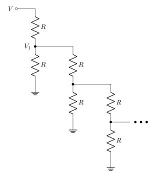
By how much does the rest of the divider chain load down the first divider? That is, in the equivalent circuit
