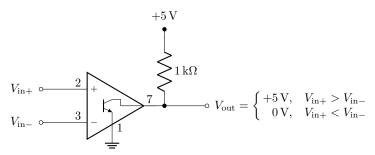
Not shown here are power-supply connections (to supplies of up to  $\pm 18 \,\mathrm{V}$ ). The inputs must stay within the supply-voltage range. To summarize the operation here:
