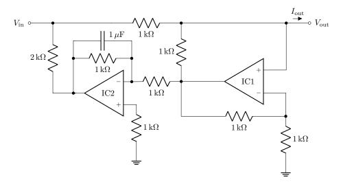
To analyze the noise here, first consider the noise contributed by the IC1 portion of the circuit. IC1 sees an input resistance of  $500 \Omega$  at the inverting input, corresponding to  $2.9 \,\mathrm{nV}/\sqrt{\mathrm{Hz}}$  of Johnson noise. The
