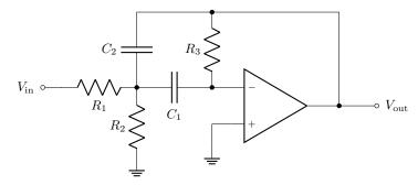
(a) Derive an expression for the gain function  $\tilde{G}(\omega)$ , and the amplitude gain function  $G(\omega)$ . Note that these are the same as the transfer function and amplitude transfer function, respectively, in the passive-filter case.
