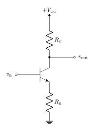
This amplifier only works as advertised on ac signals, so let's consider small ac variations v(t) and i(t) with respect to dc biases  $V_0$  and  $I_0$ , as before:
