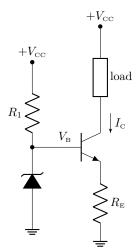
In this case, we can get a fairly coarse choice of  $V_{\rm B}$  by choosing the Zener diode, and fine-tune the current by setting  $R_{\rm E}$ .
