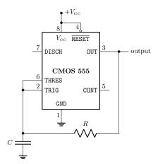
Note: this circuit only works with CMOS variants of the 555 (like the 7555), where the output will swing all the way from ground to  $+V_{CC}$ .
