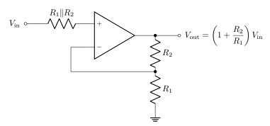
Note that the noise will be superposed with whatever the normal amplified signal will be; so this analysis will apply equally well to the bias-compensated *inverting* amplifier from Section. 7.6.1.3—the only difference is the ground and input voltages are swapped in the circuit.
