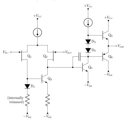
As before in Section 4.16.5, the exercise here is to identify what is going on with all the components in the schematic, based on what you know about FETs and BJTs.
