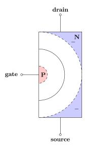
For intermediate gate voltages, the gate voltage acts as a control that modulates the resistance of the drainsource path. This acts something like modulating the flow of water in a garden hose by changing the clamping force of a pair of pliers on the hose.
