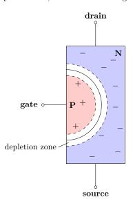
As in the semiconductor diode, a depletion zone forms at the p-n junction. In normal operation, the voltage at the gate terminal is kept below that of the drain and source, so the junction is reverse-biased. Only a small leakage current flows via the gate terminal. However, in the configuration shown, there is a low-impedance path between the drain and source terminals, through the n-type region (hence, the "n-channel").
