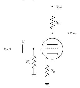
Again, due to the analogy with the JFET, the tube circuit is very similar to the JFET (common-source) amplifier shown below, which we analyzed before (Section 5.4.3).
