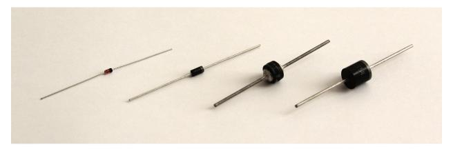
From left to right, these are: 1N914B (signal diode), 1N4001 (1-A, general-purpose rectifier), MR752 (6-A, 200-V rectifier), GI754 (6-A, 400-V rectifier). All cathodes point to the upper-right-hand corner.
