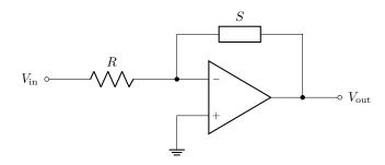
Derive an expression for  $V_{\text{out}}(t)$  in terms of an arbitrary, time-dependent input  $V_{\text{in}}(t)$ , R, and S. Assume an ideal op-amp.
