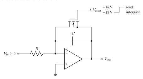
The MOSFET here acts as an analog switch, that dumps the capacitor charge when it is necessary to reset the integrator. Note that we are assuming a positive input voltage, and thus a negative output voltage. If the output voltage may have either sign, a second, reversed MOSFET may be necessary to prevent dumping the capacitor charge during integration.
