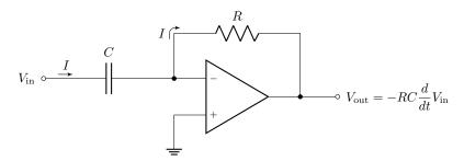
Intuitively, the current I flows in through the input, and the voltage across the capacitor is  $V_{\rm in} - V_{\rm in-} = V_{\rm in}$ , enforced by the op-amp. This same current I gets converted to a voltage, via the feedback resistor.
