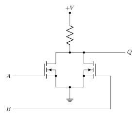
Again, either transistor can pull the output to ground, which means that either input being HIGH leads to a LOW output. A NAND gate can be made in a similar way by putting the two transistors in *series* with the resistor, so that both transistors must be activated to bring the output low. We'll see an example like this in the next section.
