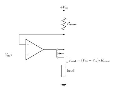
$$I_{\text{load}} = \frac{V_{\text{SS}} - V_{\text{in}}}{R_{\text{sense}}},\tag{7.137}$$
