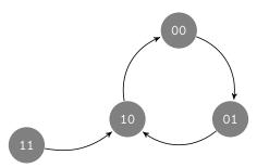
This is a directed graph of all the register states; the edges (arrows) show transitions between the states. You can use a diagram to start the design: you just begin with n flip-flops, where  $2^n$  equals or exceeds the number of distinct states. Then you use the procedure that we used for the divide-by-3 counter to generate the appropriate logic.
