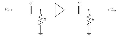
The buffer amplifier has two important properties: the input (left-hand-side connection) draws no current (and thus produces no load on the first RC filter), and the output voltage is equal to the voltage at the input.
