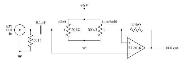
Note the ac-coupled input, a 50- $\Omega$ -terminated input (as appropriate for a 50- $\Omega$  cable connecting the clock to this circuit), and the Schmitt trigger, with TTL-compatible output. The clock offset and threshold voltages are adjustable to account for different input clock amplitudes, and to adjust the duty cycle of the resulting square wave (typically, these can both be set to  $2.5\,\mathrm{V}$ ).
