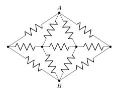
**Solution.** Notice that by symmetry, the voltage across the center resistance is zero, so the current flowing through it is zero, no matter what the voltage  $V_{AB}$ . Thus, we can remove it from the circuit. The same goes for the two other "equatorial" resistors. Thus, we have 4 parallel resistances of 2R, for a total resistance R/2.
