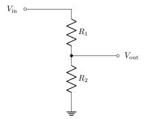
Here at the bottom of the circuit diagram, we are drawing the **ground** symbol, which means we are declaring this point to be a *fixed* voltage (say, zero), and all other voltages are *differences* with respect to ground. (In the "ground" or "earth" pin on an ac power receptacle, this is *literally* the ground outside. Often the case of electrical devices is connected to ground for safety, and in cars the entire chassis is ground.)
