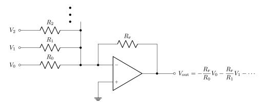
Then, for example, we can build a 4-bit DAC as in the diagram below.
