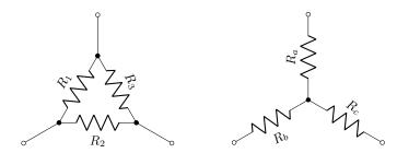
What does it mean for two resistor networks to be equivalent? Label the voltages and currents, for example, as follows.
