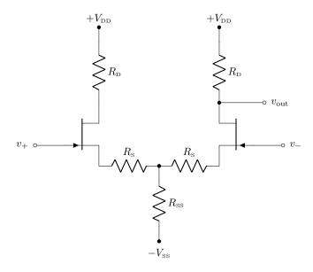
The analysis here is closely analogous to that of the BJT case, so we will only sketch the idea. Assuming a purely differential (ac) input  $\Delta v := v_+ - v_-$ , the voltage drop across  $R_{\rm ss}$  is fixed, so the two transistors act
