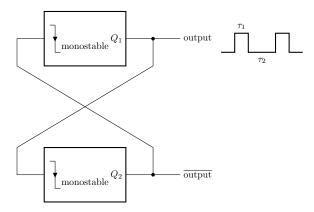
Note that the  $\tt HIGH$  and  $\tt LOW$  times are controlled separately by the durations of the two one-shots, and each one-shot triggers on the falling edge of the other.
