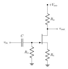
The analysis is a combination of the analysis of the grounded-source amplifier above and that of the source follower in the previous section. The result is
