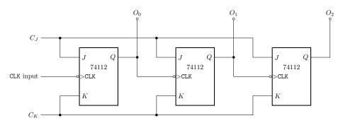
What control-input combination  $C_JC_K$  is necessary for the circuit to count, and what kind of counter is it? Describe the operation of this circuit for all other control-input combinations  $C_JC_K$ .
