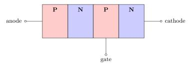
The basic operation will be something like a diode, but there is one additional "gate" connection to the internal p-type region. This is reflected in the schematic symbol, shown below.
