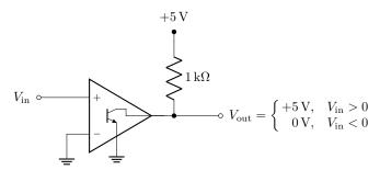
The usual output of the op-amp in the LM311 drives the base of an output transistor, whose collector is connected to the output. If  $V_{\rm in}>0$ , then the transistor acts as an open circuit, causing the output to go high to  $+5\,\rm V$  via the  $1\,\rm k\Omega$  pull-up resistor. If  $V_{\rm in}<0$ , the transistor acts as a short, causing the output to fall to zero.
