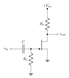
Here,  $R_{\rm G}$  maintains the dc bias of  $V_{\rm GS}$  at ground, but allows ac modulation of the gate via the capacitor C. If  $V_{\rm GS}=0$ , the quiescent current is  $I_{\rm D}=I_{\rm DSS}$ , as in the JFET current source (thus assuming that  $V_{\rm DD}$  is large enough to put the JFET into saturation). Then the output is biased at
