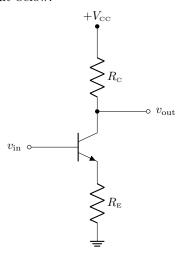
In Section 4.8, we showed the ac voltage gain of the circuit is  $G = -R_{\rm C}/R_{\rm E}$ , assuming  $\beta \gg 1$ . Rederive the ac gain of the circuit, this time **without** making any approximations involving  $\beta \gg 1$ .
