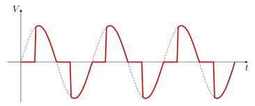
The brightness can be adjusted by changing  $R_1$ : a larger  $R_1$  leads to a longer charging time, which leads to a longer delay until the load turns on each cycle. A resulting dimmer signal is illustrated in the plot below.
