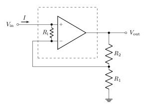
The dashed line encompasses the "real" amplifier, which consists of an ideal op-amp and a resistor modeling the input impedance. As before, the closed-loop gain (7.45) is
