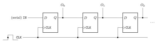
An example application is in converting serial data to parallel form (i.e., on the receiving end of a serial transmission channel). Also, note that a bit shift corresponds to a mathematical operation on binary data (divide/multiply by 2).
