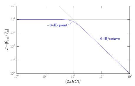
Because the integrator "passes" low frequencies without attenuation, and "rolls off" high frequencies, it is called a low-pass filter.
