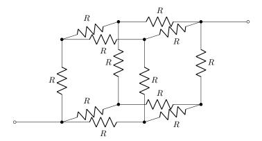
*Hint*: use symmetry, and analyze a current flowing between the two terminals. It also may (or may not) help to identify which junctions are at equivalent potentials.
