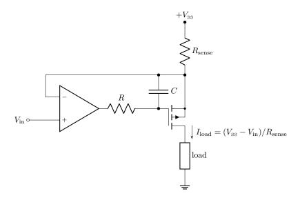
Consider a small ac signal  $v_{\rm in}$  at frequency  $\omega$  at the input (and some dc bias  $V_0$ , so  $V_{\rm in} = V_0 + v_{\rm in}$ ). Treat the FET via its transconductance  $g_{\rm m}$  (i.e.,  $i_{\rm SD} = -g_{\rm m}v_{\rm GS}$ ) and the op-amp via the finite-gain formula (7.39)
