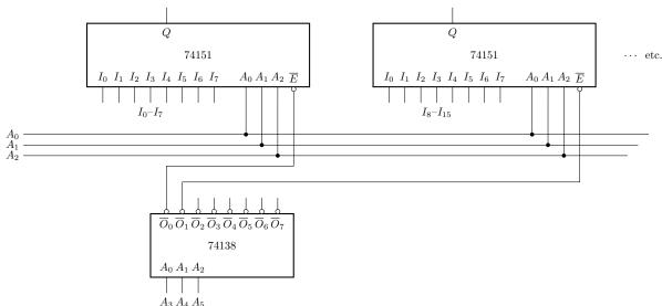
One detail that we have left out is that the Q outputs must be combined by an OR gate. An important alternative is to use chips with **three-state logic**. For these chips, the output is disconnected (high-impedance) when the chip is not enabled. In this case, you can just connect the chip outputs directly together, since only one chip will be enabled at a time. In this example, we can use the three-state alternative 74251 instead of the 74151.
