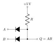
If both inputs are at +5 V then all points are at the same voltage, including the output Q. If one input is low, say A, then the situation is as shown below.
