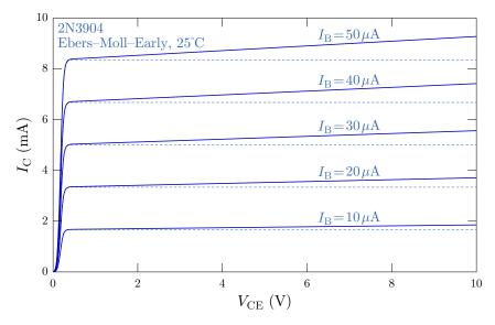
The previous Ebers–Moll curves are superimposed as dashed lines to make the difference between models more clear. The curves are no longer horizontal in the linear regime, and their changing slope means that  $\beta$  is effectively no longer independent of  $V_{\rm CE}$ . Also, the Early voltage of 90 V leads to a collector resistance of  $r_{\rm C} \approx V_{\rm AF}/I_{\rm C} \approx 20\,{\rm k}\Omega$  for the  $I_{\rm B} = 30\,\mu{\rm A}$  curve, where  $I_{\rm C} \approx 5\,{\rm mA}$ .
