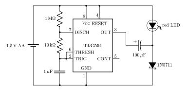
This is a standard 555 a stable multivibrator circuit (see Section 15.1), but with some adaptations to make it run and drive an LED on a  $1.5\,\mathrm{V}$  battery
