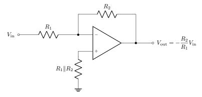
This resistor does nothing for an ideal op-amp, because no current flows through the resistor (and thus the resistor drops no voltage), but for a *real* op-amp, this trick reduces bias errors. Of course, all this assumes  $V_{\rm in}$  acts like an ideal voltage source (i.e., it has a source impedance much smaller than  $R_1$ ), otherwise the source impedance of  $V_{\rm in}$  must also enter into the compensation scheme.
