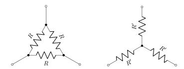
One way to do this is to redraw these circuits as the equivalent "pi" and "tee" networks below, and consider the current I into one port. However, you should *justify* that your treatment is sufficient to establish that the networks are fully equivalent.
