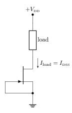
The idea is to operate the JFET in the saturation region, where  $I_{\rm D}$  is independent of  $V_{\rm DS}$ , allowing the JFET to adjust the load voltage to regulate its current. Since the gate and source are shorted (and grounded),  $V_{\rm GS} = 0$ . Then using Eq. (5.5), we find the constant current
