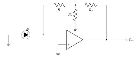
What is the effective feedback resistance R of this circuit (i.e., the resistance that makes this equivalent to the original circuit)? Find a combination of  $100 \,\mathrm{k}\Omega$  or smaller resistors that gives an effective R of  $1 \,\mathrm{G}\Omega$ .
