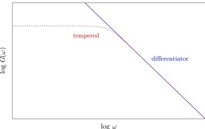
This shows the normal -6-dB scaling of the integrator as the solid line, with the dashed line showing the "tempered" behavior with the feedback resistor rolling off the low-frequency gain.
