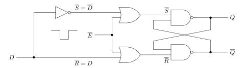
Here we changed notation so that the clock signal is now an "enable-low" ( $\overline{E}$ ), and the flip-flop now accepts input only when  $\overline{E} = \texttt{LOW}$ . To keep things compact, we will refer to this circuit with the small block diagram below.
