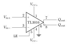
This comparator has both regular and inverted outputs, and the outputs are TTL-compatible. To summarize the regular operation:
