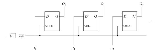
Once latched, the register holds the output state, independent of the inputs, until the next clock pulse. One application is where a shared set of data logic lines drives several devices; a register at the input of each device can hold the relevant logic data for each particular device while the data lines drive other devices.
