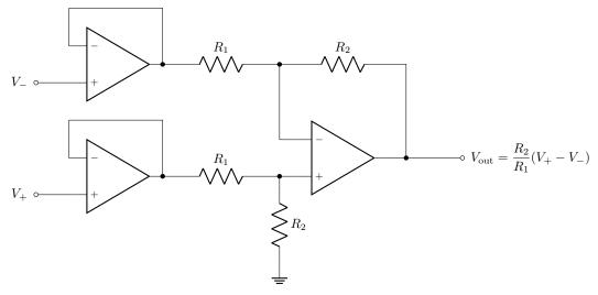
The point is that this entire circuit should come in a single package, with laser-trimmed (matched) resistor networks, for good performance and to make life easy. This also guarantees that any errors in the matched resistor pairs due to temperature drifts is kept to a minimum.
