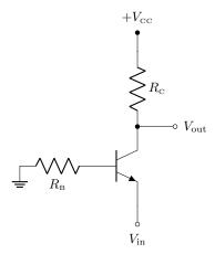
(a) Consider small voltage changes  $v_{\rm in}$  and  $v_{\rm out}$  at the input and output (i.e., ignore bias voltages). Compute the voltage gain  $G = v_{\rm out}/v_{\rm in}$ .
