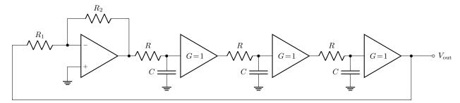
Note that the first op-amp is connected as an inverting amplifier, and the output  $V_{\text{out}}$  feeds back into the inverting amplifier. There are 3 RC filters in the feedback loop. The oscillation condition is that the phase shift of each RC filter is  $60^{\circ}$ , so the total RC phase shift is  $180^{\circ}$ . In combination with the action of the inverting amplifier, this is a total phase of  $0^{\circ}$ , which means that we have positive feedback.
