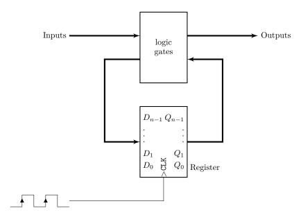
Again, the basic idea is to use a register to hold logic values, the outputs of which are transformed and fed back to the register inputs via a logic-array block. Here we will discuss implementing the logic-array block in a very general way by replacing it with memory, either RAM or ROM. In the ROM case, the state machine is suited for fixed operation (e.g., as a counter), whereas with RAM we have the possibility that the state machine can adapt to input and even reprogram itself.
