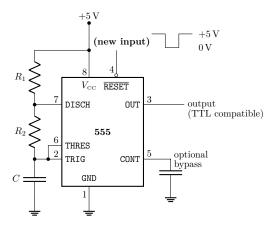
Describe what happens when the  $\overline{\text{RESET}}$  input goes through one HIGH-LOW-HIGH pulse cycle as shown. More specifically, you should say what happens to the OUT line and capacitor voltage on each transition (HIGH-LOW and LOW-HIGH), and what happens after the input pulse is finished.
