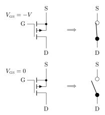
Again the current to be switched flows from source to drain. A zero gate voltage (with respect to the source, which is now drawn as the upper terminal) still causes the "switch" to be open. To close the MOSFET switch, a *negative* gate voltage (again, with respect to the source, so  $V_{\rm GS} < 0$ ) is required to close the gate.
