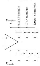
Here the large  $470 - \mu F$  capacitor acts as a large charge reservoir, as appropriate for the high-current circuit, but only responds well at relatively low frequencies due to a high intrinsic inductance. Progressively smaller capacitors with lower inductance will help stabilize the power-supply voltage at higher frequencies. In this case, the smallest capacitors should be located closest to the op-amp, with the location of the large capacitors not so critical.
