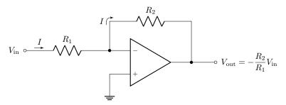
To analyze this circuit, assume a current I flows into the input. Golden rule 2 says that the inverting-input voltage  $V_{\rm in-}$  must be zero, so
