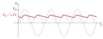
Again, we lose almost another volt compared to the half-wave rectifier, but for the same load and filter capacitor, we get much less ripple. Yet better power supplies (with smaller ripple) can be realized by adding a linear regulator IC.
