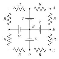
Give the Thévenin-equivalent circuit for the circuit in the diagram, as seen between
