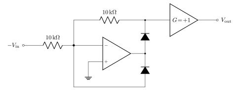
Note that the second circuit takes the *inverted* signal  $-V_{in}$  instead of  $V_{in}$ , which could be implemented by another inverting amplifier that is not shown.
