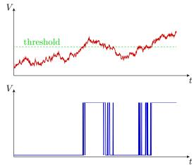
Ideally, with a noise-free signal, the output (shown in the bottom plot) would have one up transition, then later a down transition, and then an up transition again, instead of the many clustered around the three "ideal" trigger times.
