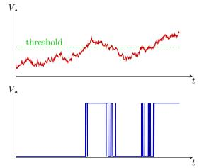
But what we see is that due to the noise, the output signal makes many (spurious) transitions whenever the signal crosses a reference, whereas we would expect a smooth input signal to make only one transition at each crossing.
