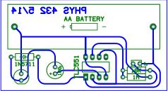
Note that the copper layer is mirrored from this point of view; again, you can tell from the text. In a professionally fabricated board (i.e., not the kind you do yourself), these labels would be silk-screened onto the component side over a (typically green) protective layer, called the "solder mask."
