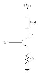
In this case, the transistor is maintaining the collector current  $I_{\rm c}$ . To see that this works, note that the base and emitter voltages are related as usual by
