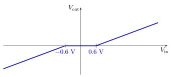
The problem in using this as an amplifier is that it leads to **crossover distortion**, because the base-emitter drop changes as the signal crosses through zero. If you put a relatively large (compared to 0.6 V) sine wave into the input, the output shows the crossover distortion whenever the signal is crossing through zero.
