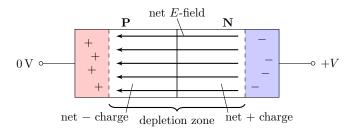
In this case, the electric field due to the applied voltage *adds* with the electric field from the carrier diffusion. This also pulls the p-type carriers towards the anode (the terminal on the p-type material), and n-type carriers towards the cathode. The net effect is just to *increase* the width of the depletion zone.
