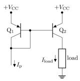
Suppose that  $Q_1$  is at temperature  $T_1$  and  $Q_2$  is at temperature  $T_2$  (in class we assumed these were the same). Derive an expression for the current  $I_{load}$  in terms of the program current  $I_p$  and the temperatures. Assume that the transistors are otherwise identical.
