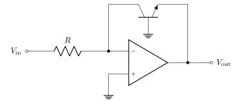
*Hint:* the function of the transistor, as in the inverting amplifier, is to convert a current into a voltage, so use an appropriate relation to describe the transistor.
