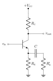
At ac frequencies the emitter resistance is  $R_{\rm E} || R'_{\rm E}$  (which is just  $R'_{\rm E}$  if  $R'_{\rm E} \ll R_{\rm E}$ ). This circuit allows the amount of emitter degeneration to be set independently at ac and dc by choosing the two resistors appropriately.
