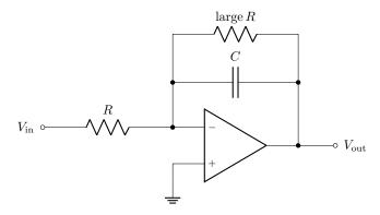
The feedback network then defines an RC frequency (a small frequency, since the resistance is large), below which the resistor dominates the feedback impedance, and the op-amp acts as an inverting amplifier. This levels the low-frequency gain to some finite value, as illustrated schematically below.
