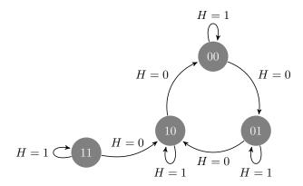
In addition, as an example output bit, we will define a "zero" output bit Z to be 1 if the counter's output bit is 00, and is 0 otherwise.
