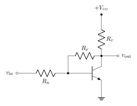
*Hint*: first solve the circuit without resistor  $R_{\rm F}$  in the circuit, then adapt your solution to the case where  $R_{\rm F}$  is present.
