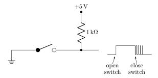
That is, if the switch is open, the output is pulled up by the resistor to +5 V, while a closed switch corresponds to a 0-V output.
