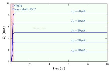
The major remaining defect of this plot is that the curves are essentially horizontal in the linear regime, which indicates a divergent collector resistance  $r_c$ ; this is the next correction to consider below.
