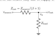
Again, from this point of view, the transistor is "lumped into" the source circuit, which is appropriate because it is acting as a linear device.
