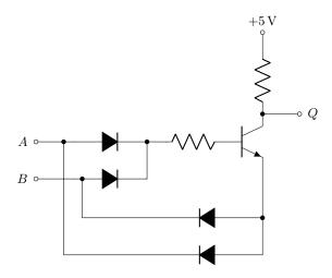
**Solution.** Due to the arrangement of diodes, the only way to turn the transistor ON is to have one input HIGH and one LOW. In this case, the output is LOW; otherwise the output is HIGH. Thus, this is an XNOR gate.
