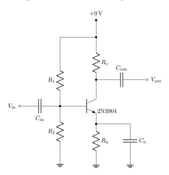
The design criteria for this amplifier are: a large gain over a usable bandwidth of  $100\,\mathrm{Hz}{-}20\,\mathrm{kHz}$ , an input impedance of  $10\,\mathrm{k}\Omega$ , a quiescent current (dc current) of  $100\,\mu\mathrm{A}$  (dominated by the collector current). The dynamic range of the output should also be reasonably close to the maximum possible, so we will fix the collector voltage at  $+V_{\mathrm{CC}}/2$ . Also assume an ideality value of n=1.09 for the 2N3904.
