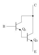
Assume transistor  $Q_1$  has parameters  $\beta_1$ ,  $V_{BE1}$ ,  $r_{e1}$ ,  $h_{oe1}$ , etc., while  $Q_2$  has parameters  $\beta_2$ ,  $V_{BE2}$ ,  $r_{e2}$ ,  $h_{oe2}$ , etc.
