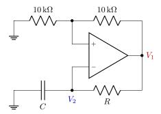
Here, the amplifier is standard op-amp, acting as a comparator in open-loop mode. We will assume the output rails are  $+V_{\text{max}}$  and  $-V_{\text{max}}$ . There is a 50% voltage divider feeding the noninverting input, similar to the Schmitt trigger above. This sets the trigger points of the comparator to  $+V_{\text{max}}/2$  and  $-V_{\text{max}}/2$ .
