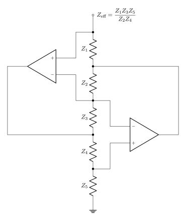
(a) Show that the effective input impedance is as advertised. Begin by considering a voltage V and a current I at the input terminal, and divide them to obtain the impedance.
