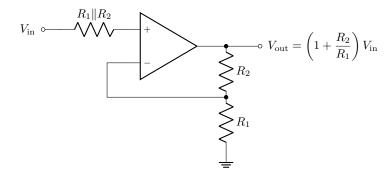
Balancing input impedances is a bit trickier for ac-coupled amplifiers. A good example is shown below.
