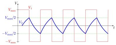
If the output  $V_1$  is positive, the RC circuit charges  $V_2$  until the inverting-input voltage exceeds the  $V_{\text{max}+}/2$  trigger point, at which point  $V_1$  goes negative, and the charging proceeds in the opposite direction until  $V_2$  reaches  $V_{\text{max}-}/2$ , and the cycle repeats.
