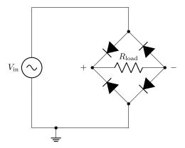
This passes both the positive and negative peaks, as shown below. Trace the current through the diodes on both phases of the input to convince yourself that this works out.
