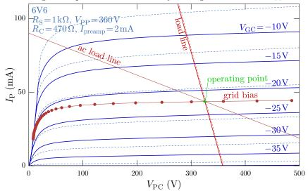
The (dc) load curve is plotted from Eq. (6.46); the dashed counterpart is the load line obtained by ignoring the small contribution of  $I_s$ . Clearly the screen current makes a difference, but here it doesn't change much to ignore it.
