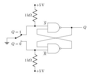
During a bounce, the switch makes no connection to either contact, so both  $\overline{S}$  and  $\overline{R}$  are 1. This is the memory state, so the flip-flop holds the last switch state, which persists through the duration of the bouncing.
