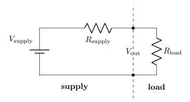
This is just a voltage divider, so we can write the output as
