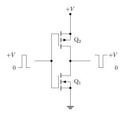
With a zero input,  $Q_1$  is OFF and  $Q_2$  is ON, so the output is pulled (actively) up to +V. With a positive input, the transistors exchange states, so the output is pulled (actively) down to ground.
