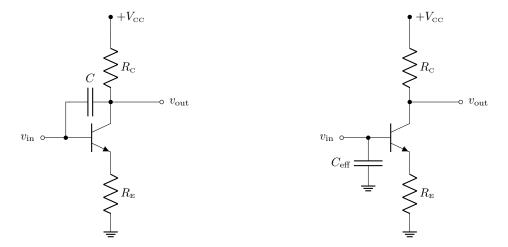
The reason that the Miller capacitance is a serious problem in a high-gain circuit is that seen as an effective input capacitance  $C_{\rm eff}$  as shown in the right-hand diagram, the effective capacitance is
