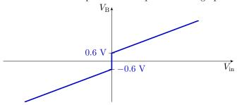
This response combined with the crossover distortion results in, in principle, a distortion-free output.
