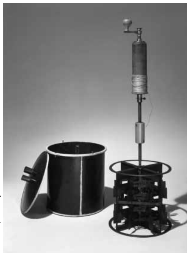
Figure 2.6 Joule used this apparatus to measure what was once called the “mechanical equivalent of heat.”
