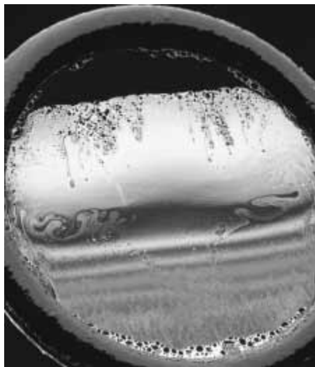
Figure 22.3 A film has two surfaces and so requires twice the force to increase its size.
