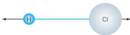
Figure 14.23 The single vibration of HCl has the hydrogen and chlorine atoms moving alternately back and forth. The hydrogen’s movement is much larger than the chlorine’s, because of H’s much higher mass.
