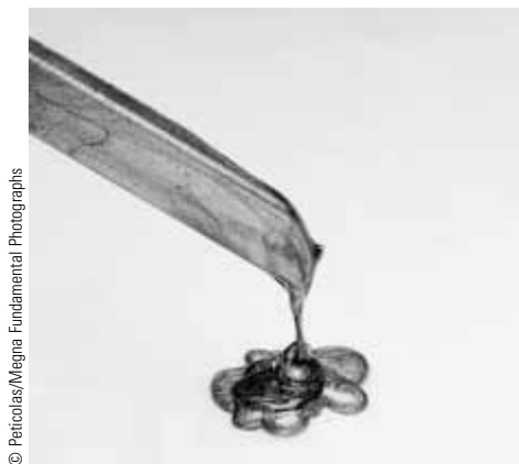
Figure 21.1 Amorphous or glassy materials, like the ones shown, have randomly arranged molecules. Crystalline materials, on the other hand, are solids that are built up of units that repeat in three dimensions.
