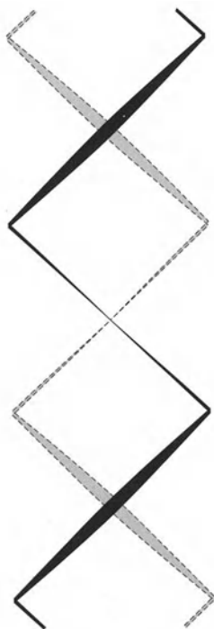
Fig. 12.13 When the grey and black helices intersect they are at right angles to each other. The two helices, one corresponding to a helical molecule and the other to a transition occurring perpendicular to the molecular helix, are of opposite hand.
